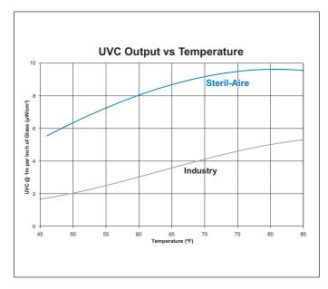
Steril-Aire's multi-patented UVC Emitter provides the best and longest-lasting UVC performance available. As shown in the comparison graph *(above)*, it has been independently tested to deliver up to 6 times the output of other ultraviolet devices under HVAC operating conditions (50 °F @ 400 fpm air velocity).
